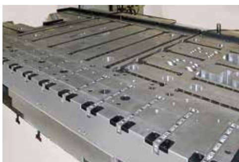
Roller bars with hydraulic lifting integrated in a press bed
